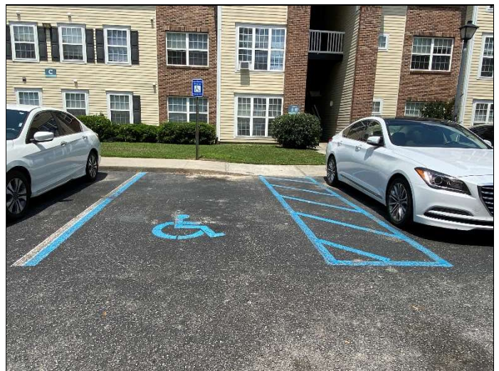
114. Several accessible stall access aisles less than 60" in width
